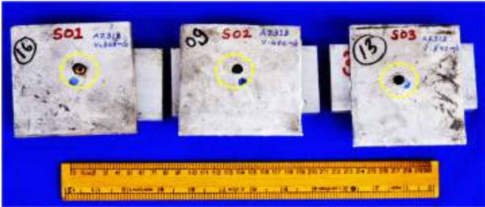
Figure 16. Ballistic test of AZ31B base metal with three different velocities.
