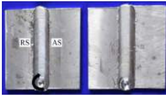
Fig. 2 Defect-free AZ31B friction stir welds
