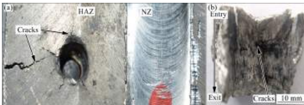
Fig. 7 Damage images of front side and cross-section of HAZ-PWHT target plate after ballistic test: (a) Front view; (b) Crater path of projectile
