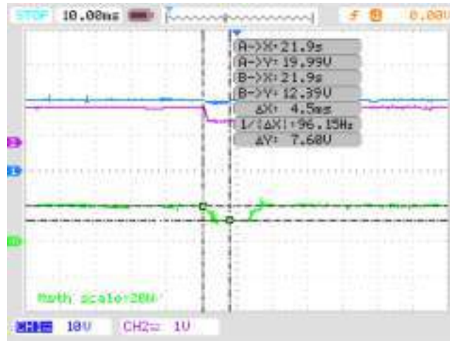
Fig. 9. Current, voltage and power profile during shading condition with bypass diode.
