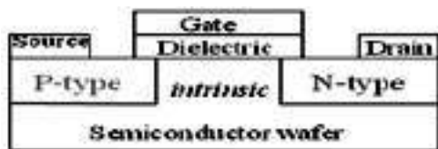
Figure 1. Basic Structure of TFET
