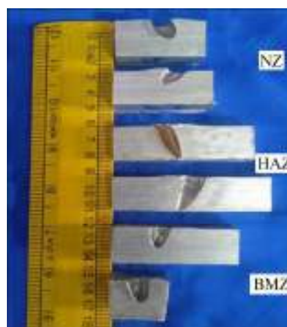
Fig. 9 Penetration channels of Al6062 backing plates after ballistic tests
